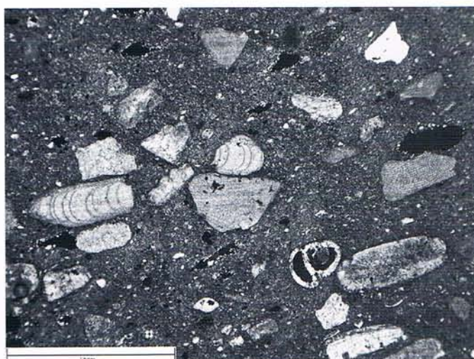
9 Cross polarized image of Memphite LBA Canaanite jar sample (225/B), note Amphiroa algae clasts in centre and centre left. The scale bar is 1 mm long.
